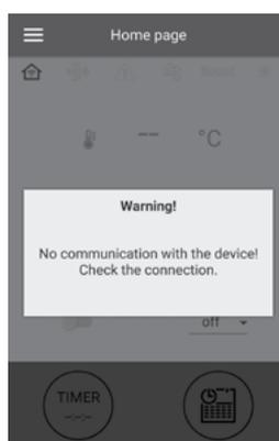
After installing the application, connect the mobile device to the unit as to a Wi-Fi access point (**FAN: + 16 characters of the ID number**) indicated on the control board and on the unit casing.
