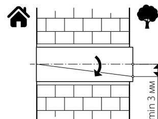
**4.** Fill the spaces between the air ducts and the wall with a mounting foam through the specially designed holes in the mounting template.
