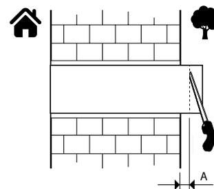
**3.** Fix the mounting template on the wall to install the air ducts.
