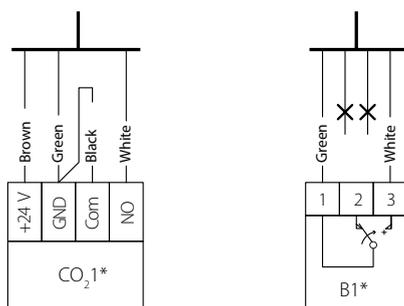
Connecting humidity sensor or CO<sub>2</sub> sensor to the control unit via a cable, which is attached to the bracket
