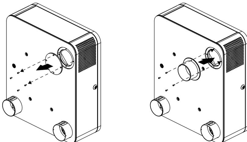
**6. Caution! Install the condensate preheater before fixing the unit to the wall (see the Installation manual of the heater).**
