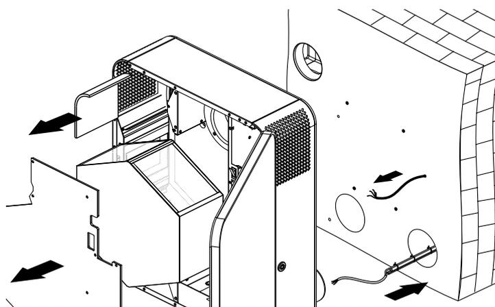
**7.** Install the outer ventilation hood:
