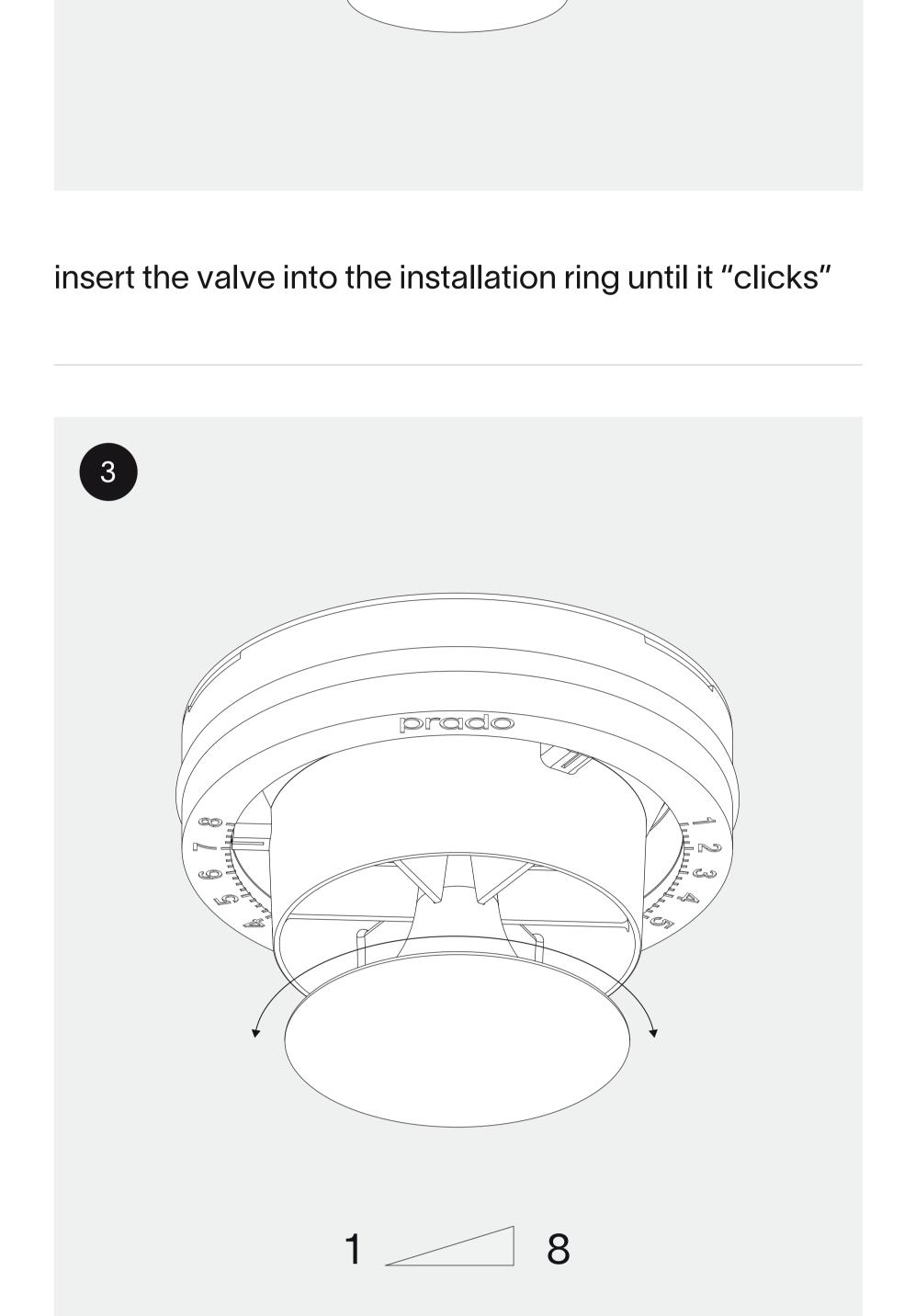
twist the luminaire to adjust the ventilation flow level
